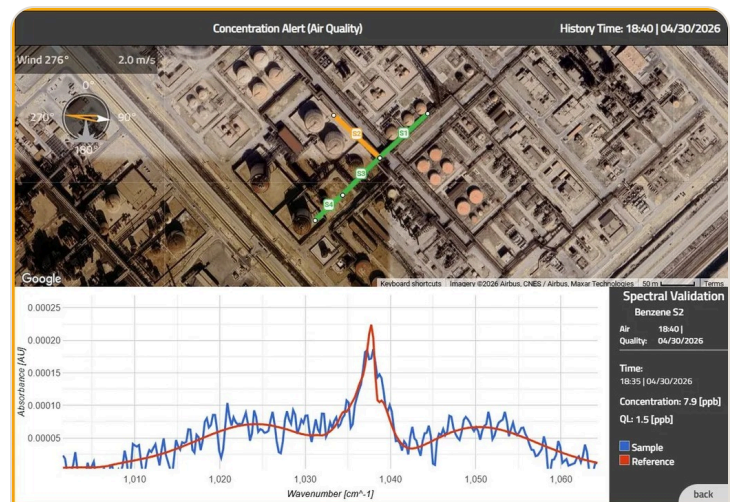
Source location and spectral validation, live in the platform — a benzene event on path S2.
